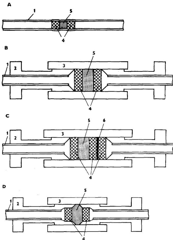
Fig. 3A—D. Scheme of adsorption element, models A—D: 1 = PTFE capillary of 1.0 mm I.D.; 2 = PTFE connector outlet; 3 = polyethylene tube of 3 mm I.D.; 4 = porous polypropylene disc; 5 = microgranular affinity adsorbent; 6 = cellulose acetate microporous membrane for electrophoresis (placed in the system closer to the outlet valve).
