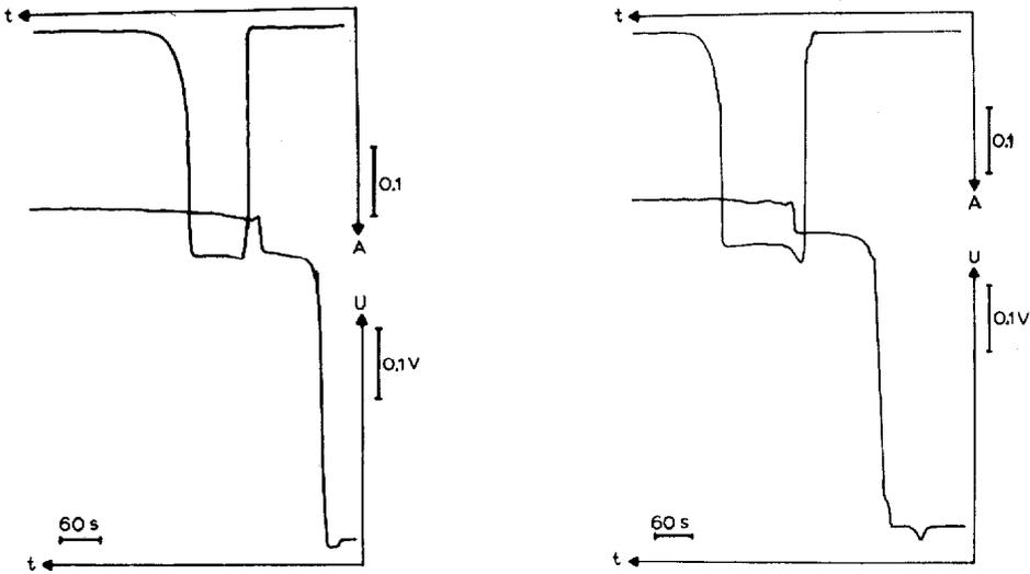
Fig. 6. Control analysis of ligate (isotachopheric standard of MMAbT) in the absence of the adsorption element in electrolyte system I (see Table II). Sample, 5  $\mu$ l of 1% solution of MMAbT in phosphate-buffered saline containing 0.1% sodium azide applied via a septum; current intensity 50  $\mu$ A, during detection 20  $\mu$ A; temperature 20°C.
